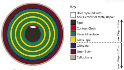
This Full Pipe Repair can be carried out with the UPS 11000 'A' Kit. This kit contains all the items needed to repair any size pipe up to 1600 psi. Please contact Unique Polymer Systems LTD for further details:
